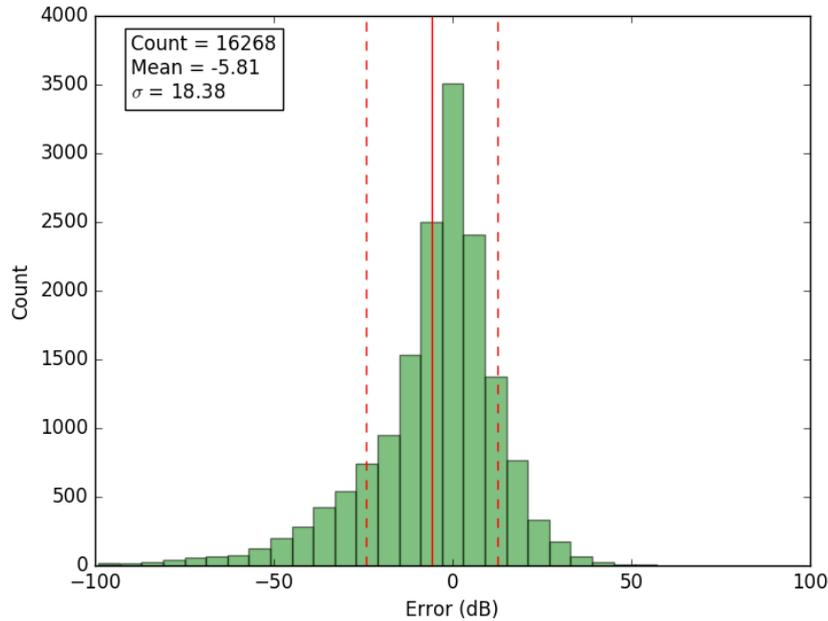
Figure 2: Predicted vs. Measured Field Strength
