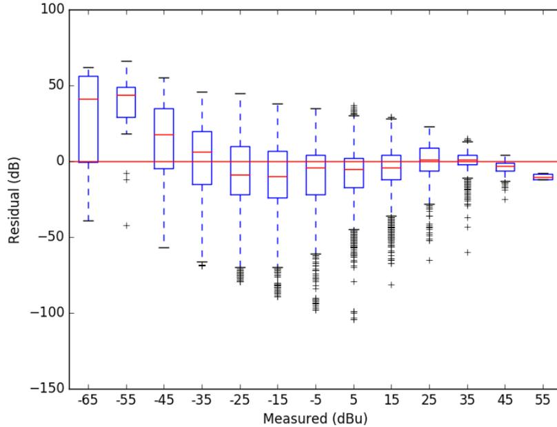
Figure 3: Residual Distribution vs. Measured Field Strength
